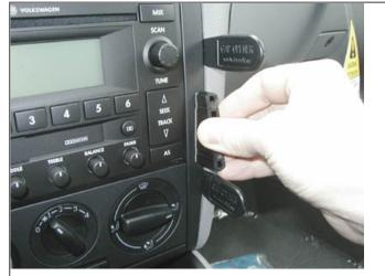
2. Press the angled edge firmly into the gap and at the same time: bend Part 1 to the left so the angled edge hooks behind the console edge panel. Press forward on Part 1. so the adhesive tape attaches to the center console panel. Pull out the gap openers.
