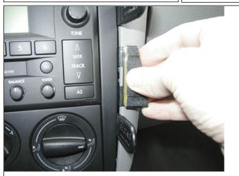
1. This ProClip consists of two parts:Part 1: The attaching part (the smallest part). Part 2: The ProClip faceplate (the big part with holes). Press the thin end of the enclosed gap openers into the gap between the center console panel and the console edge, to widen the gap. Peel off the cover of the adhesive tape on Part 1. Place the angled edge on Part 1 in the exact same position as in the picture, in the same height, so the angled edge is into the gap between the gap openers.
